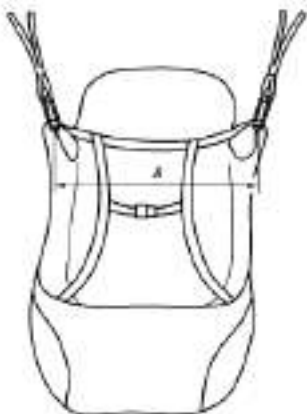
Figure 5 — Width of harness attachment points
