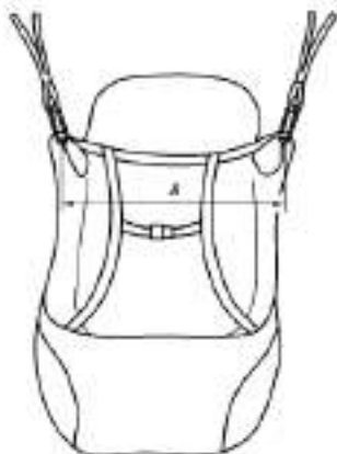
Figure 5 — Width of harness attachment points
